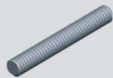
of case hardening steel C15, thread rolled, profile quality 7e (average) according to DIN 103, pitch tolerance (for 300 mm) length  $\pm 0,3$  mm
